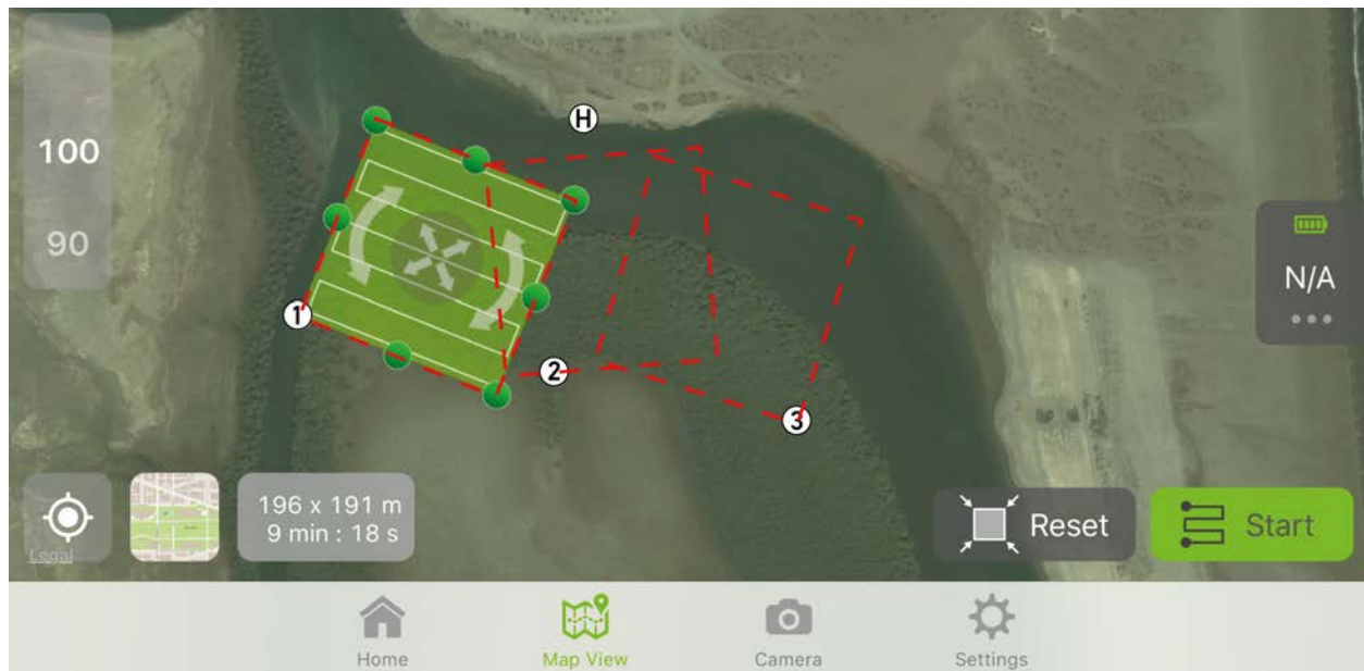
Figure 10. Mission plan for the Northern part of Khor Kalba Ramsar Site in Fujairah (three missions shown and Home point H)
