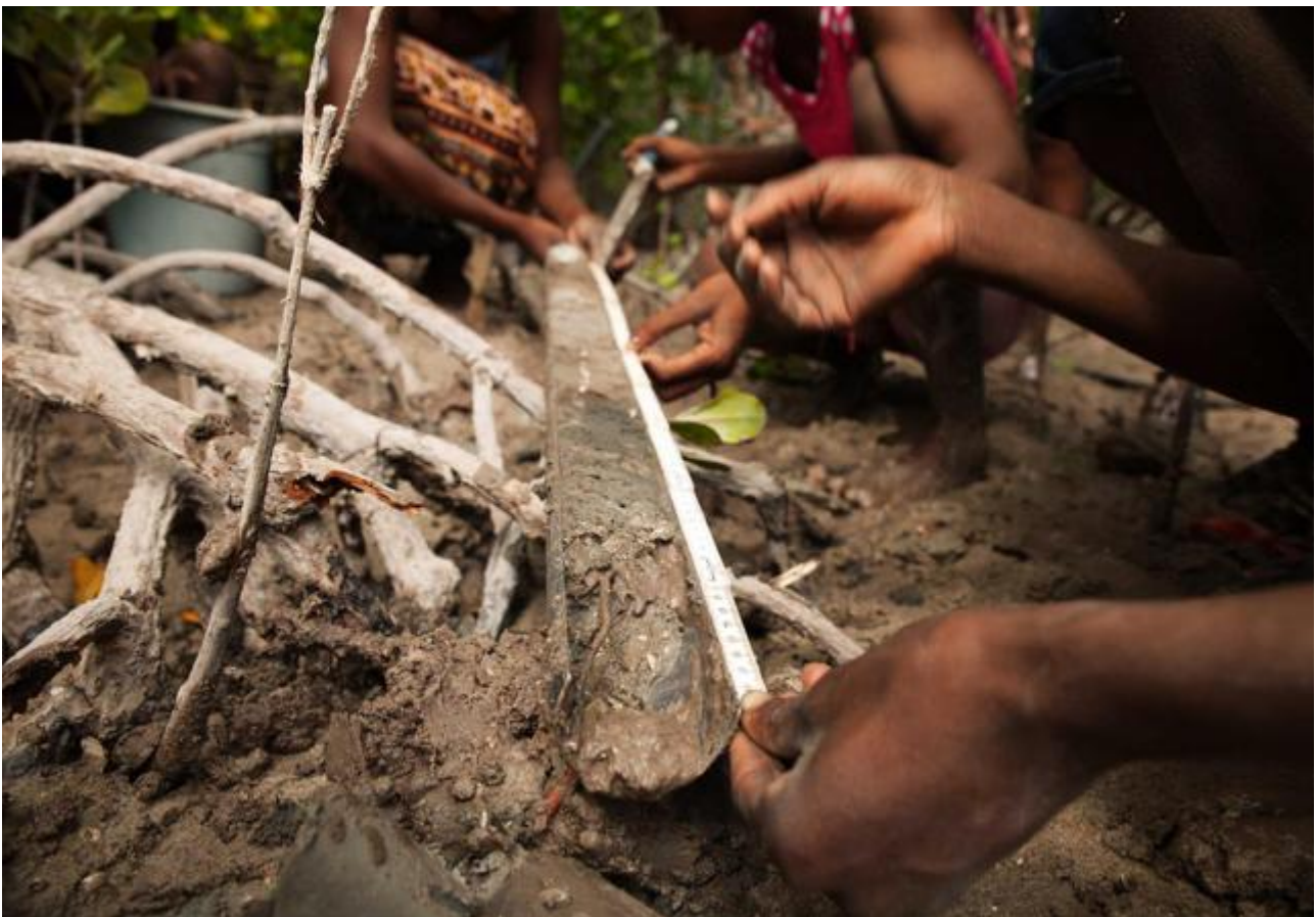
A sediment core is examined as part of Blue Carbon field research in Madagascar (image credit and © Garth Cripps, Blue Ventures).
